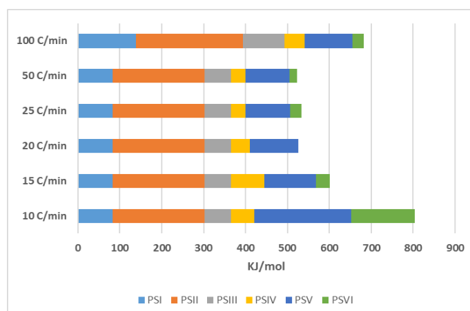
Figure 19 Comparison of activation energies obtained after modelling of pyrolysis for six pseudo components (Program temperature is used for comparison, 60-80 mesh Q. cerris cork was used)
