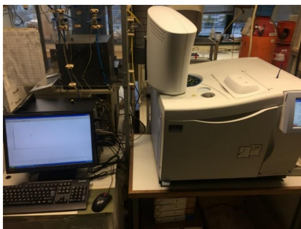
Figure 47 Perkin-Elmer Clarus 680 gas chromatograph
